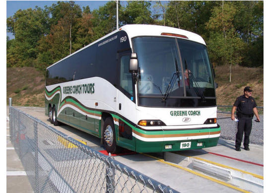
Motor coach entering the PBBT at the Greene County Inspection Station, Bulls Gap, Tennessee.
